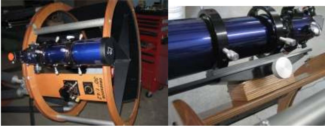
The mounting hardware, scope and eyepiece work perfect as a counterweight. No additional weight is needed, at either end of the scope. The cage is much easier to handle, and I’ve got a great finder to boot!
