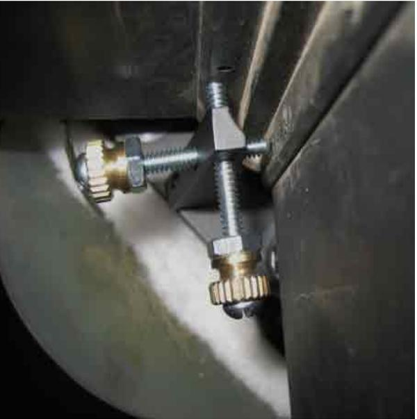
Closeup of rotation adjustment screws
