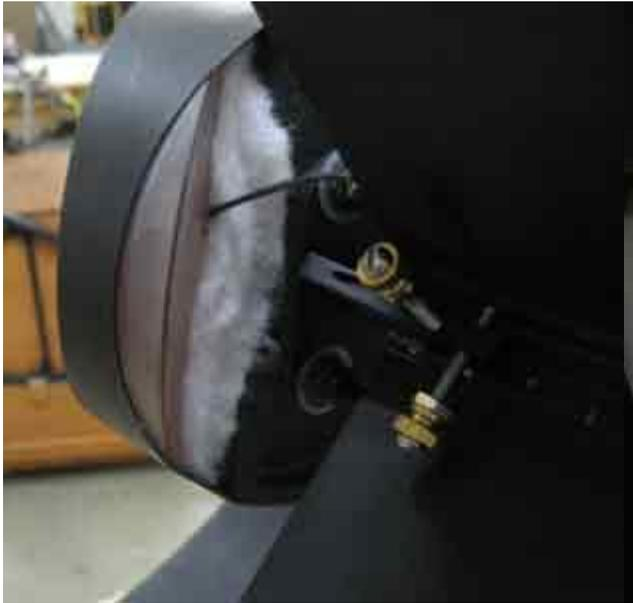
Secondary holder installed into spider
