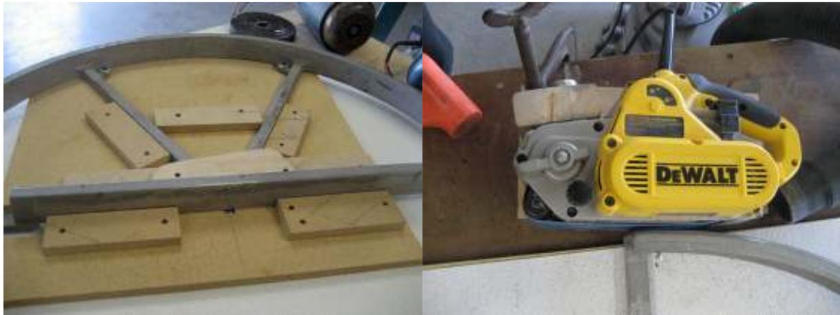
The photo on the left shows the jig that held the bearing. You can see the pivot bolt recessed in the jig. This pivot determines the center of the radius of curvature of the bearing. I took some time to position the bearing in the jig as precisely as possible.
