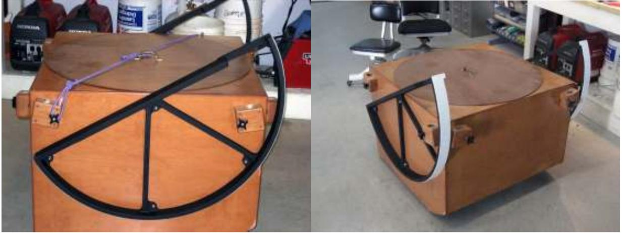
I've used the scope since making these mods. The bearings work great. I do not see any way, nor do I see a need to improve on them. My attempt to install a ServoCat system before the mod was a failure. After the mods things are working great with good to excellent pointing and tracking.
