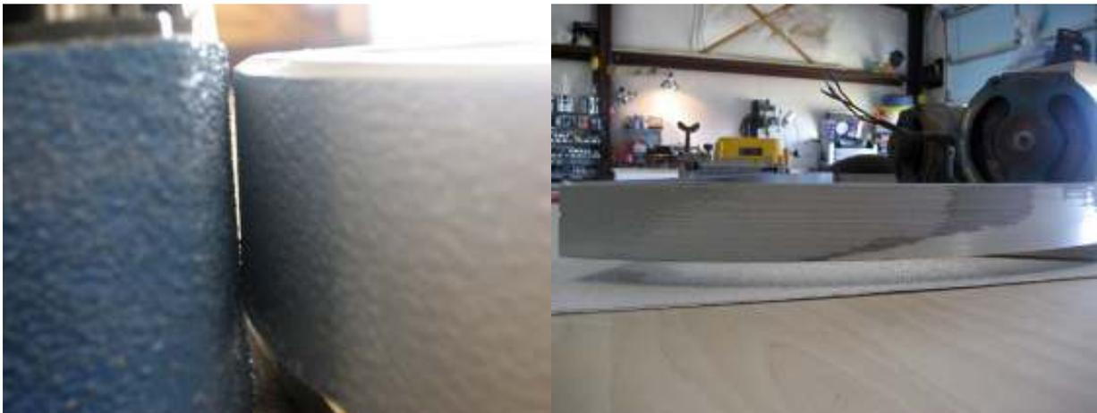
The photo on the right below shows the warp in the bearing. There are two areas of strong contact with an area of minimal contact between. In fact the two areas of contact are high spots with low spots on either side of each of them. The motors on the jig are being used as counter weights to make sure the jig does not tip or tilt. The bearing is rotated away from the belt-sander for the photo. In action it rotates against the blue belt.
