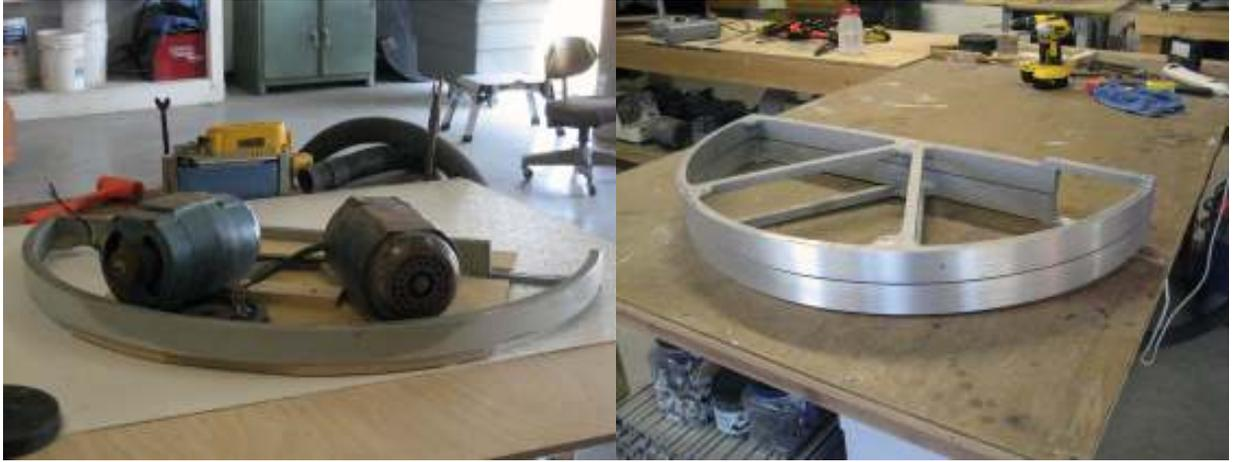
New glass-board could be applied once the bearings were trued. I epoxied over sized strips on the bearing surface. The strips were then held in place with ratcheting straps as shown in the left photo below. This held the glass-board very tightly against the bearing. After a couple of days curing time I used a trim router to cut away the extra glass-board. It was a messy job, as seen in the photo below right.
